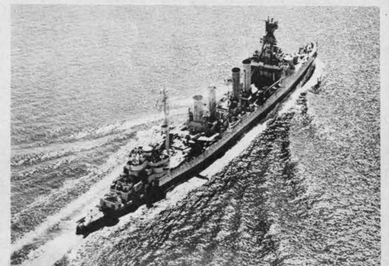
Four stacks rise between dispersed superstructure groups of Omahas, oldest U. S. CL's. Guns are carried in casemats and two turrets.
